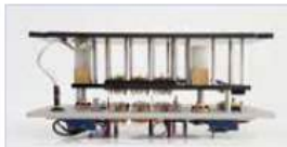
ICT fixture for Parsec RF-20 handler (pneumatic, offline)
